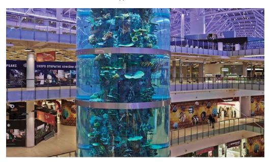
The aquarium at the Avia Park shopping center in Moscow is 75 feet tall. The tank is constructed of seven sections of R-Cast® acrylic, which weigh up to 26,000 pounds each. The acrylic is up to eight inces thick to retain the 98,000 gallons of water within the tank.
